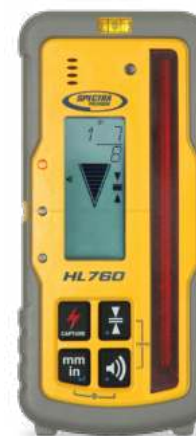
HL760 Laserometer to measure and display beam location
